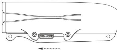
**Switch-Off:** Slide the switch to the tail of the camera to switch it off, and the indicators will all go out.
