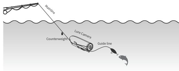
After the camera is connected, you can troll normally. If you troll faster, it is recommended to add a counterweight on the main line (as shown in the figure) to ensure that the camera will not float up when the speed is high. The counterweight can be adjusted according to your preset trolling speed.
