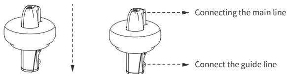
2. Attach the camera to the fishing line as shown.
